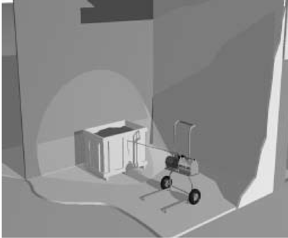
Figure-2: ISOCS Performing Assay on a Waste Container
